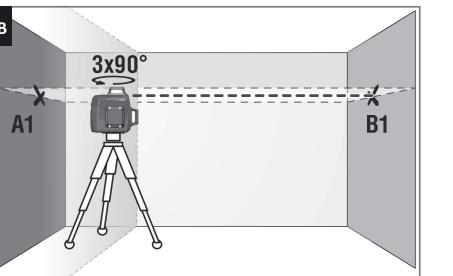
3. Repeat actions described in point 2 twice, rotating the laser level in one direction.
