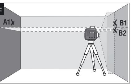
5. Rotate the laser level by 180° and mark location of laser lines crossing on the opposite wall as A2 (points A1, A2 must be located at the same vertical) (Figure D).
