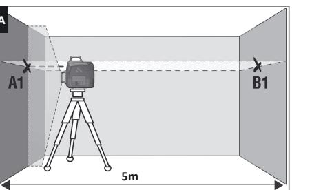
2. Rotate the laser level by 90°, measure deviation of a laser line from point B1 (Figure B). If deviation exceeds 1.5 mm – please contact the service center.
